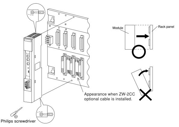
This module can be installed in any one of the optional slots. Be careful not to bend the connector pins on the module by applying too much force to them. Optional slots have each port numbers. When an error occurs, the JW50H/70H/100H (control module) stores the port number corresponding to the error occurred module into system memory #050 in the PC. This is applied only error code 53: Optional error.
