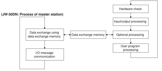
The JW-50DN receives responses from all slave stations. If not, after a communication time out, it will complete one I/O message communication cycle, and exchange data with the JW50H/70H/100H control module.
