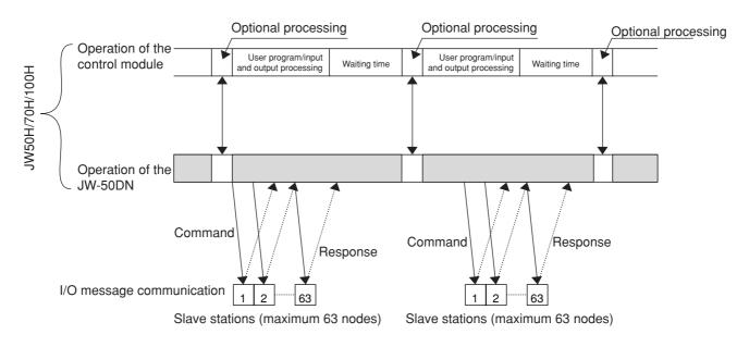
Note: The synchronous calculation operation is only possible with one module, including other communication modules (JW-10CM, JW-20CM). Therefore, be careful because using multiple modules in the synchronous mode may not permit synchronous operation.
