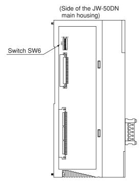
(2) Install the JW-50DN into a rack panel using the two attachment screws. Before installation or removal, make sure to shut OFF the power supply to the PC.
