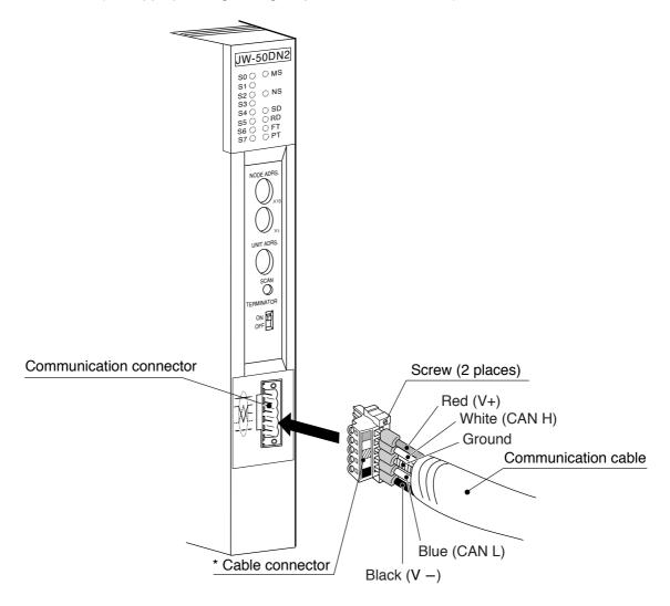
\* One male connector is supplied with the JW-50DN2. Model name: MSTB2.5/5-STF-5.08AUM (made by Phoenix Contact )
