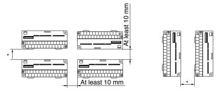
\* Secure the space that is needed to run cables
