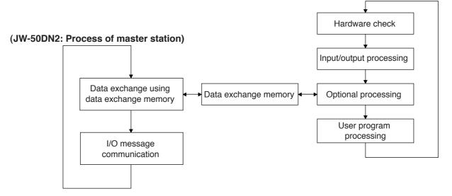
The JW-50DN2 receives responses from all slave stations. If not, after a communication time out, it will complete one I/O message communication cycle, and exchange data with the JW50H/70H/100H control module.
