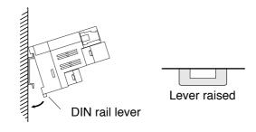
(2) To remove the slave module from the DIN rails, press down the groove in the DIN rail lever using a slotted screwdriver and lift the slave module up to remove it.
