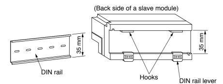
① Put the hooks on the back of the slave module on the DIN rail and press in the direction shown by the arrow.
