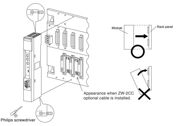
This module can be installed in any one of the optional slots. Be careful not to bend the connector pins on the module by applying too much force to them. Optional slots have each port numbers. When an error occurs, the JW50H/70H/100H (control module) stores the port number corresponding to the error occurred module into system memory #050 in the PLC.
