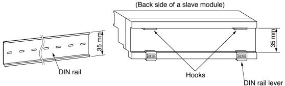
(1) Put the hooks on the back of the slave module on the DIN rail and press in the direction shown by the arrow.
