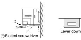
③ Install mounting brackets on a DIN rail
