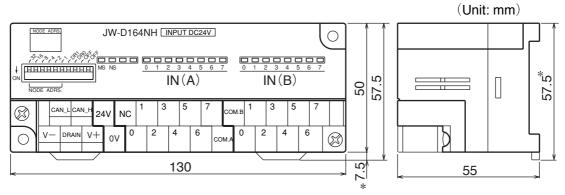
\* Dimensions when the DIN rail lever is slid in.
