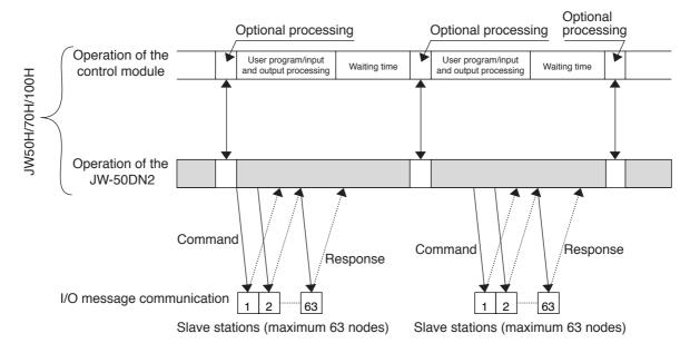
Note: The synchronous calculation operation is only possible with one module, including other communication modules (JW-10CM, JW-20CM). Therefore, be careful because using multiple modules in the synchronous mode may not be supported proper synchronous operation.
