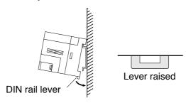
(2) To remove the slave module from the DIN rails, press down the groove in the DIN rail lever using a slotted screwdriver and lift the slave module up to remove it.
