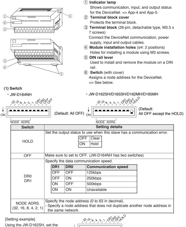
Using the JW-D162SH, set the output status to use when an error occurs to "HOLD," set the communication speed to 125 kbps, and assign node address 10.
