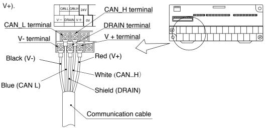
One set of communication cable consists of 5 lines. Thick and thin cables are available.
