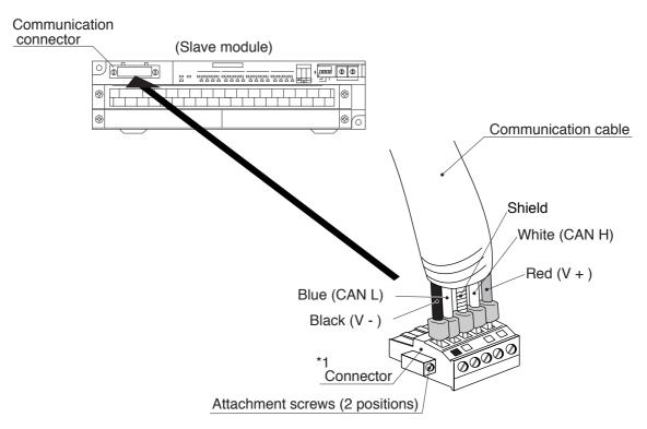
\*1: One communication cable connector is supplied with each slave module. Connector model: MVSTBR2.5/5-STF-5.08 AUM (made by Phoenix contact)
