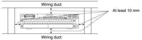
If more than one slave module is installed, allow the following distance between them.
