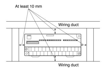
If more than one slave module is installed, allow the following distance between them.
