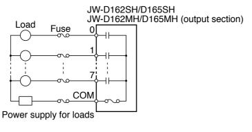
If a fuse blows, find the cause (short circuit in the external wiring, load exceeds the rated output, etc.), correct the situation and then replace the fuse.
