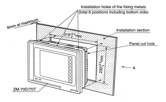
② Insert the fixing metals(6 pieces) supplied with the control terminal into installation holes(6 positions) of the body. Tighten the retention screws of the fixing metal to fix the control terminal on an installtion section of the panel.
