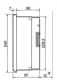
\*Leave a minimum of 50mm for wiring the link connection cable and printer connection cable. (on the back of the main housing)
