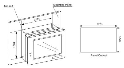
2. Insert 4 pieces of the fixtures attached to ZM-62E into the mounting holes on ZM-62E. Tighten them with the locking screws.
