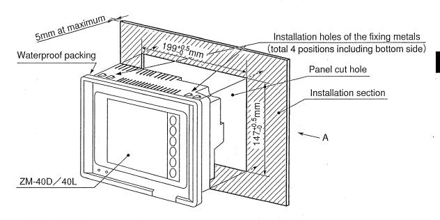
② Insert the fixing metals (4 pieces) supplied with the Control Terminal into installation holes (4 positions) of the body. Tighten the retention screws of the fixing metal to fix the Control Terminal on an installation section of the panel.
