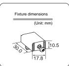
\* When the ZM-300 unit is attached to the mounting panel, the fixtures and frame grounds (FG) are connected. To prevent static electricity, be sure to connect the mounting panel to the frame ground.
