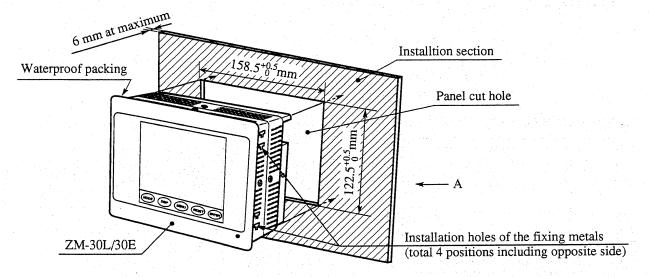
② Insert the fixing metals (4 pieces) supplied with the Control Terminal into installation holes (4 positions) of the body. Tighten the retention screws of the fixing metal to fix the Control Terminal on an installation section of the panel.
