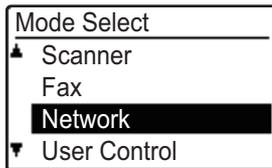
Select "Network" with the [▼] or [▲] key, and press the [OK] key.
