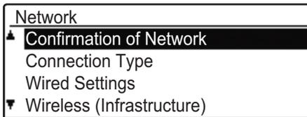
Select "Confirmation of Network" with the [▼] or [▲] key, and press the [OK] key.
