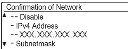
Show and check the IP address with the [▼] or [▲] key.
