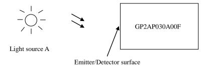
Illuminance should be measured and evaluated at Emitter/Detector surface of GP2AP030A00F.
