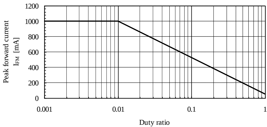
Fig.3 Peak forward current vs. duty ratio
