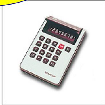
1973: World's first calculator with an LCD display
