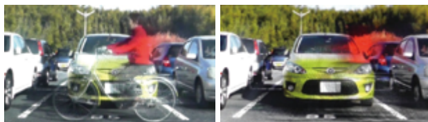
Display at −30°C SFR LCD (left) and normal LCD (right)
