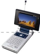
Sharp released the industry's first cycloid style mobile phone with LCD capable of swiveling 90-degrees, able to receive One Seg terrestrial digital TV broadcasts. The AQUOS mobile phone became highly popular for its use of Sharp's LCD technology developed for LCD TVs.
