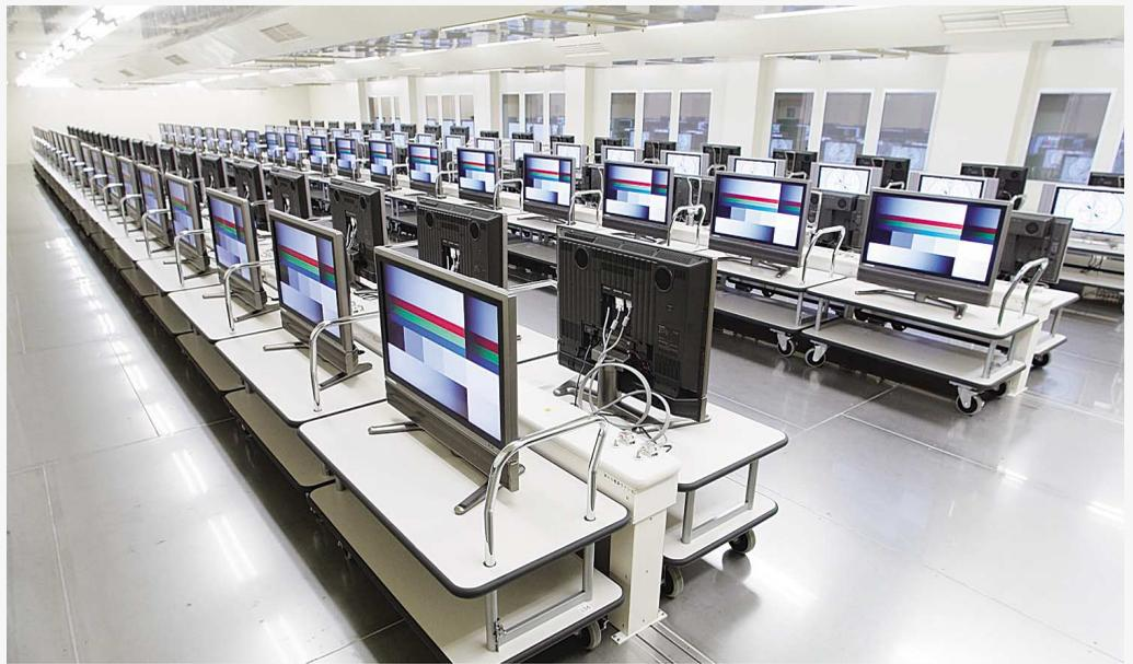
LCD TV production line (isothermal test process)
