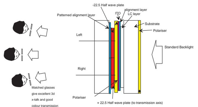
Fig. 8 Internal polariser 3d display.
