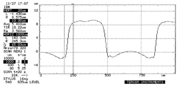
Fig. 4 Profile measurement of commercial retarder stripes.
