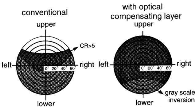
Fig. 3 The effect of optical compensating layer to the viewing angle.
