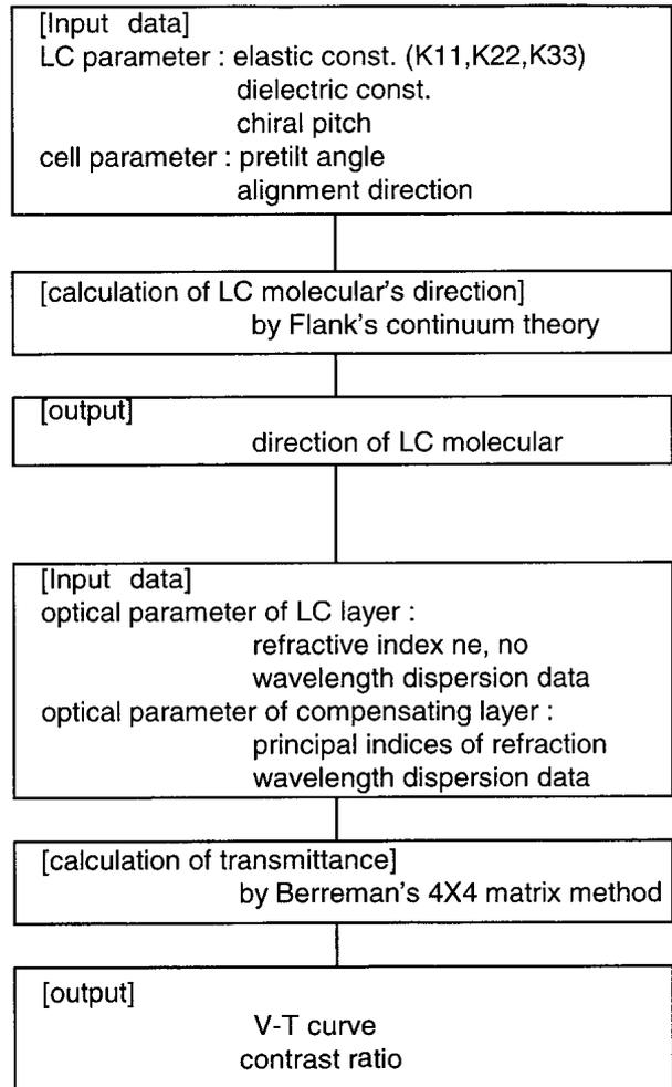
Fig. 1 Simulation flow.
