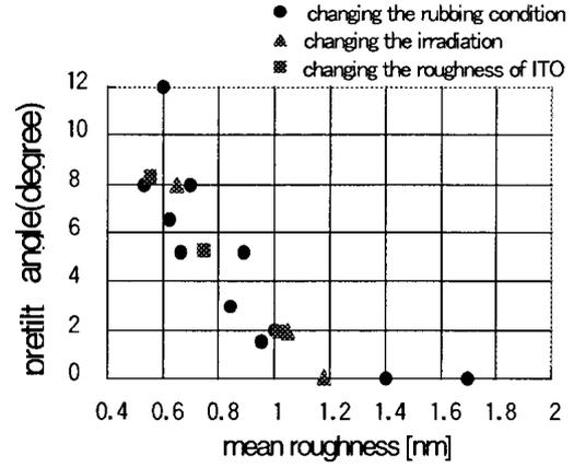
Fig. 7 Relation between mean roughness and pretilt angle.
