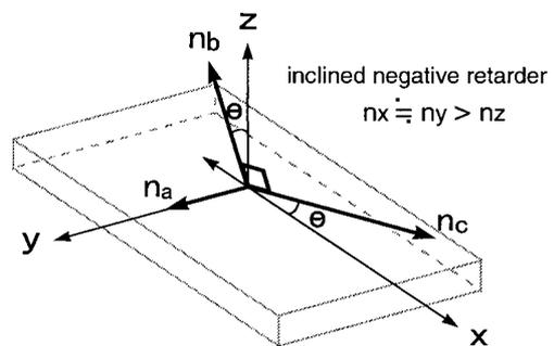
Fig. 2 The image of the refractive index ellipsoid of optical compensating layer.
