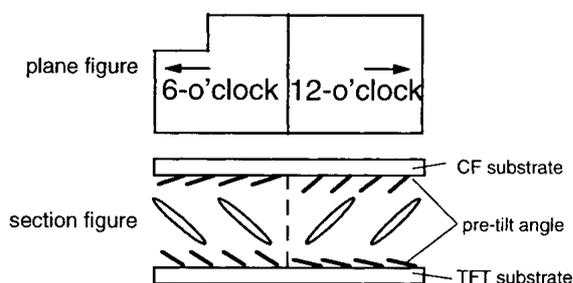
Fig. 5 Two-domain LCD structure.
