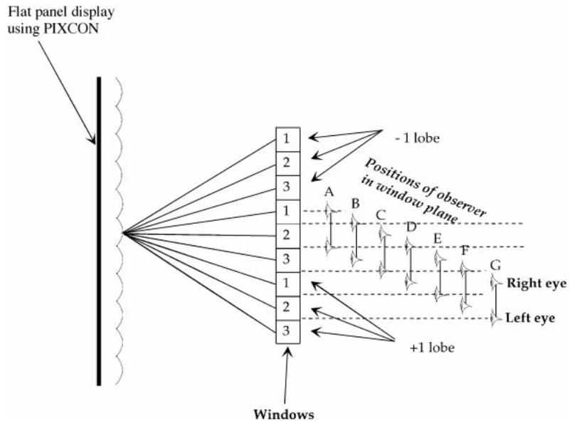
Fig. 8 Electronic tracking using PIXCON display.
