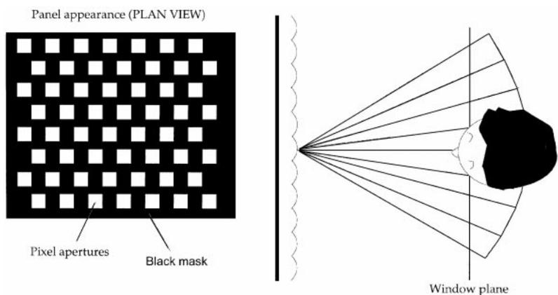
Fig. 7 Flat panel autostereoscopic display using novel PIXCON pixel configuration.
