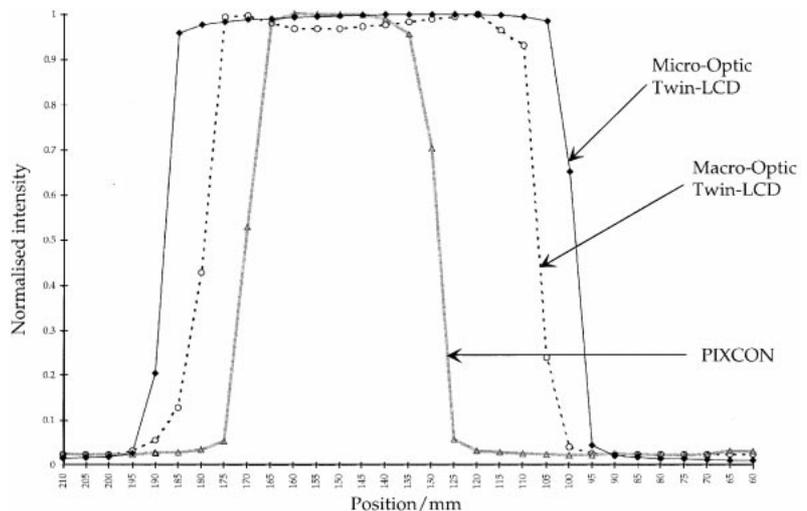
**Fig. 4** Window profiles for the illuminators used in Macro-Optic Twin-LCD Micro-Optic Twin-LCD and PIXCON displays.
