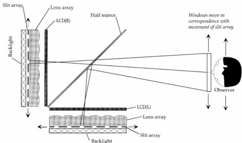
**Fig. 3** The Micro-Optic Twin-LCD display.
