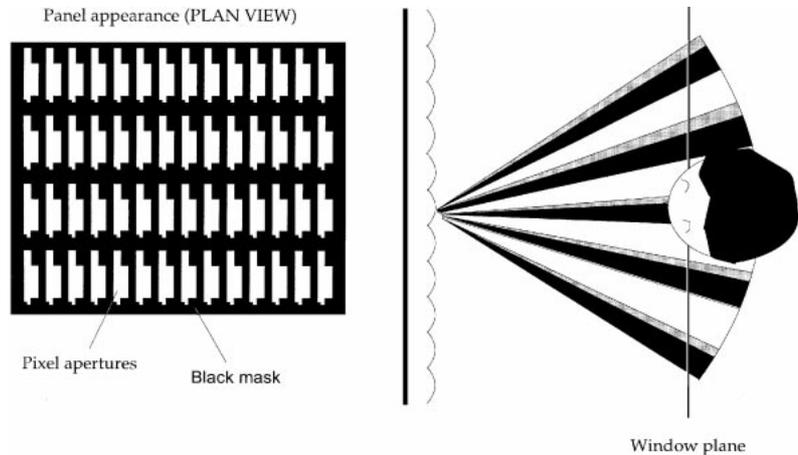
Fig. 6 Flat panel autostereoscopic display using Sharp LQ10M211.
