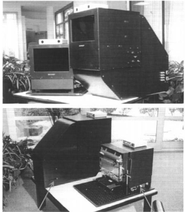
Fig. 5 Comparison of display sizes for Macro-Optic and Micro-Optic Twin-LCD displays
