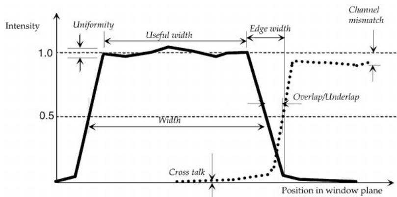
**Fig. 2** Degradation of window quality.
