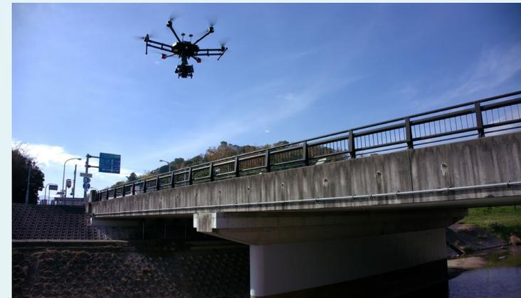
8K-camera drone on an aerial inspection
