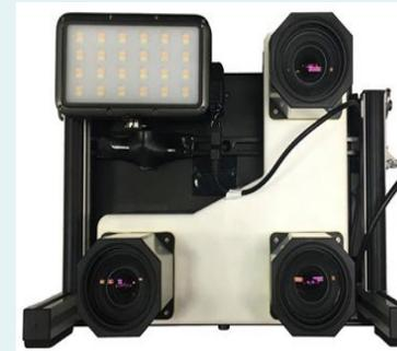
Triplet-lens camera rebar arrangement inspection system
