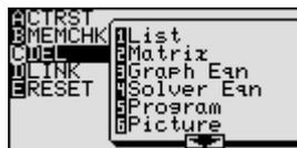
The calculator can execute calculation of inverse matrix and matrix multiplication. A system of linear equations can be solved easily using the Matrix feature.
