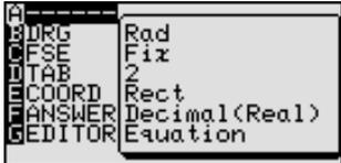
Specify two figures after the decimal point on the set up screen.
