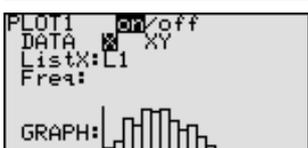
Input of the specified values for drawing a histogram from the list L1 of the statistical quantity has been completed.
